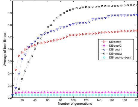
**Fig. 2.** Average of best fitness values of 30 independent runs for each of the five types of mutation operators tested in this work (see Section 2), using 500 individuals and 200 generations, to maximise energy consumption from electric vehicles' batteries (Equation 7). Higher values are preferred.
