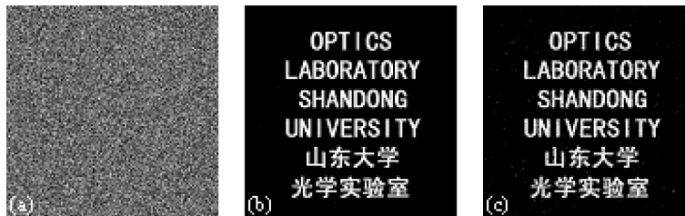
Figure 1. Simulation results of phase-only image encryption: (a) transmitted phase map; (b) retrieved binary image by using the correct G_2 at the right position; (c) retrieved binary image from a 400×400-pixel section of the image shown in (a).
