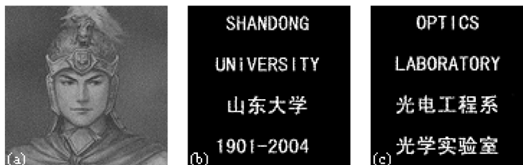
Figure 3. Double-image encryption and watermarking with one set of interferograms embedded in four different host images: (a) One of the four transmitted watermarked images; (b) and (c) retrieved binary images with different G_2 .
