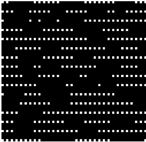
Fig. 4 Input signal for the interaction height experiments that simulates a portion of the LCD panel with arbitrary pixels turned on or off.
