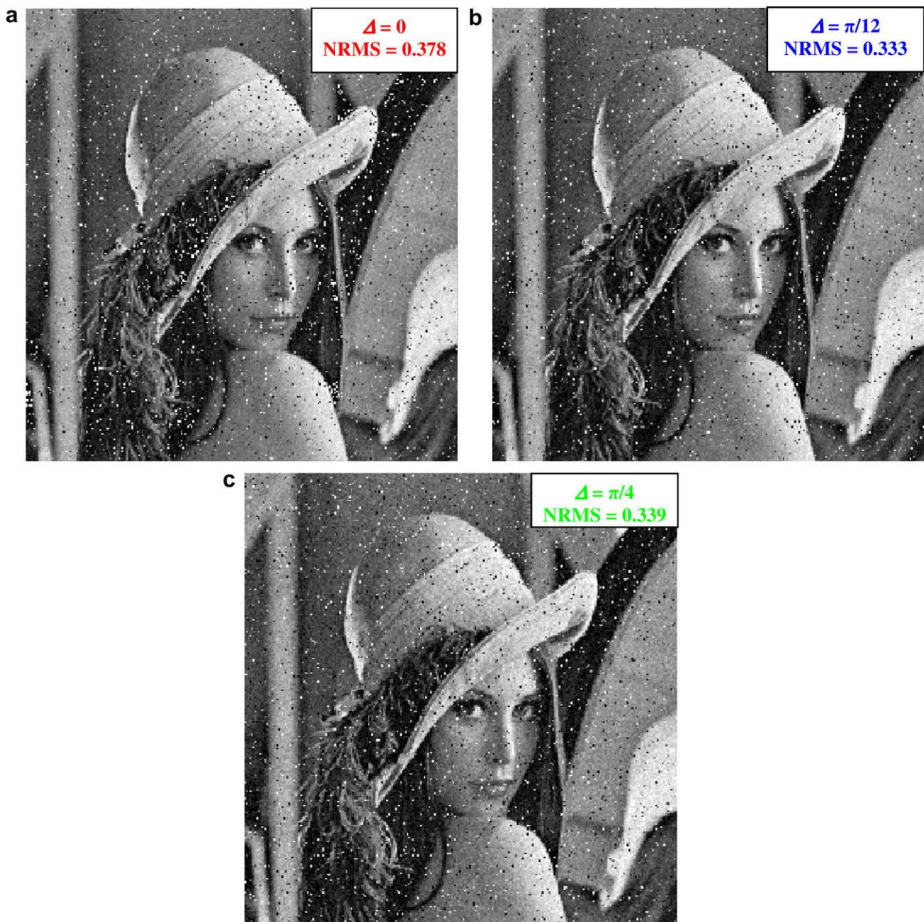
Fig. 8. With 10% of the pixels in error, as in indicated in Fig 5c. Noisy decrypted images for three cases: \Delta = (a) 0, (b) \pi/12 , and (c) \pi/4 .
