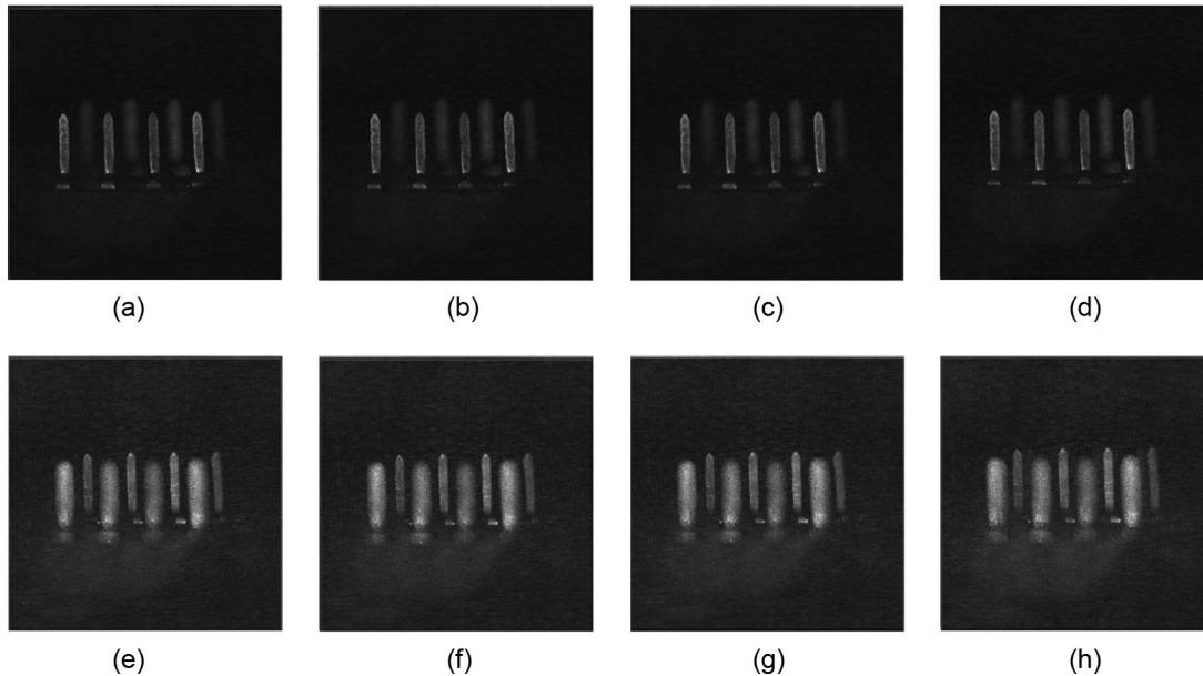
Fig. 5. Depth effects from low compressed data. (a)–(d) Reconstructions from the original, JPEG2000, quantized, and SPIHT coded data, respectively, for reconstruction distance 263 mm. (e)–(h) Same for distance 277 mm.
