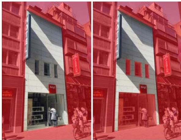
Figure 2: Reference data collection: façade area (left) and façade without windows and doors (right).
