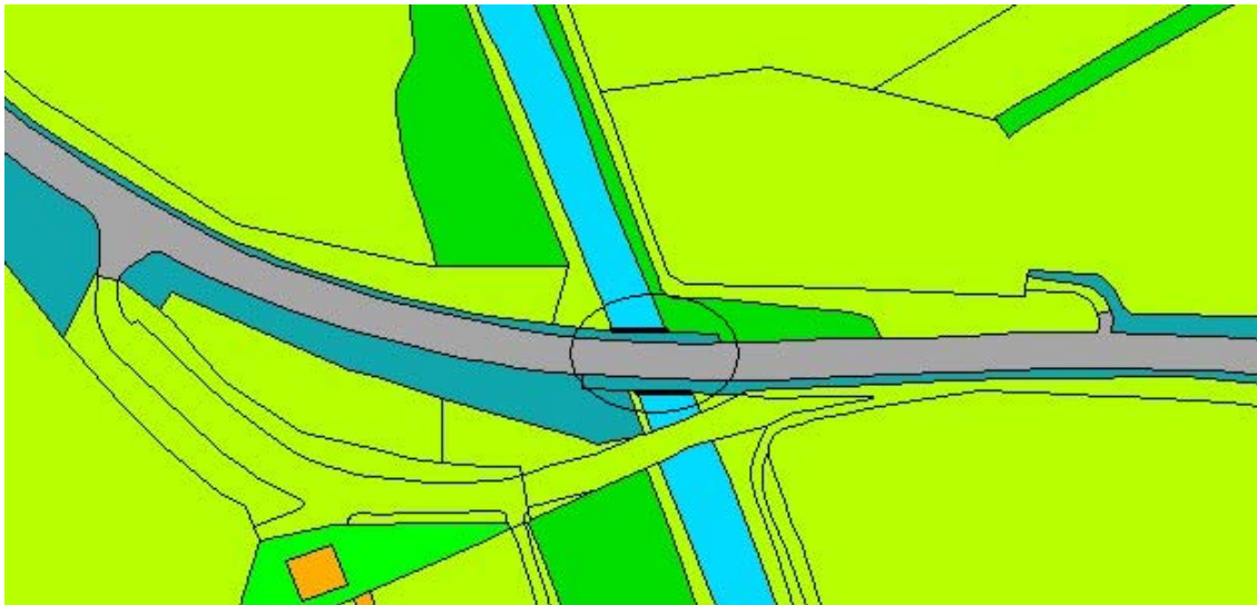
Figure 1. A river (running top to bottom) is segmented by a road (running left to right). The edges of the occlusion are highlighted.
