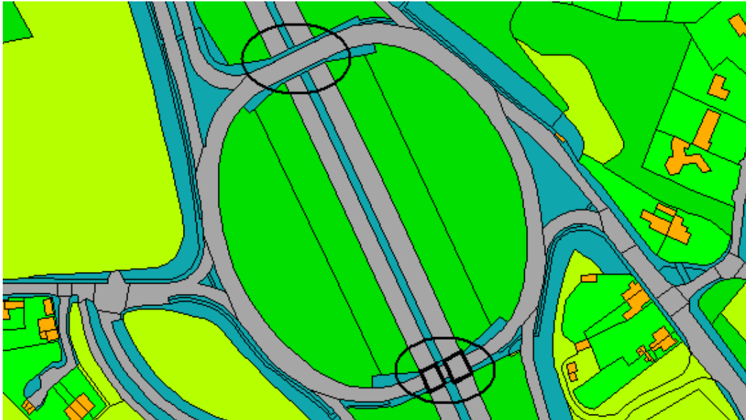
Figure 2. The road running from top to bottom was originally segmented by the roundabout (depicted on top of this figure). Adding additional “occluded” road segments (highlighted at the bottom of this figure) reconnects the original road segments.
