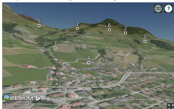
Figure 2: 3D Georeferencing platform. The volunteer digitizes correspondences in the image and the virtual globe.
